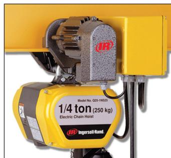
*Motorized Trolley Suspension*
